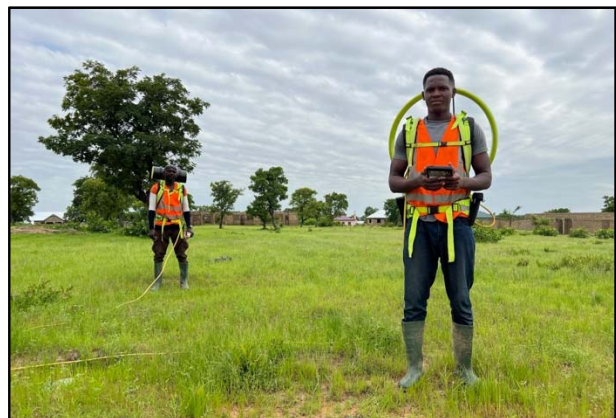
Photo 2: Castle technicians about to start another day’s Loupe EM geophysical survey.
